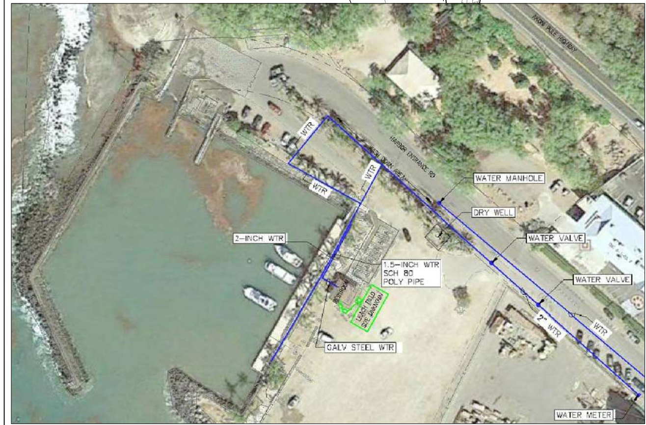
WATER METER & WATER VALVE LOCATIONS
