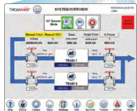
The PLC-based controller combines sophisticated system operation and reporting with an operator-friendly, touch screen display.
